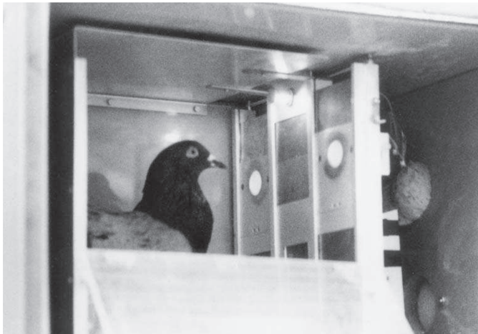
FIG. 9.1. A two-key operant chamber for birds. Schedules of food reinforcement are arranged simultaneously on each key. Author Photo.
